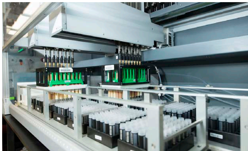
Figure 1: Tecan Freedom Evo 200 – customized to perform positive pressure SPE-based fractionation of the crude extracts. The methodology is fully automated and capable of processing 88 extracts in a single run to generate 616 fractions in under three hours. The fractions are dried, weighed and then plated on 384-well plates suitable for biological testing.
